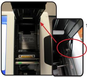
Using the barrel key open the front panel. If the ballot is easily accessible, gently pull it out. Be careful not to rip the card and leave any pieces in the unit. Release the hinge on the right side by gently pulling it forward before lowering the door. Close and lock the door. If not, proceed to step 2.
