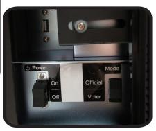
If it still cannot be removed open the side panel access door and turn the unit off.
