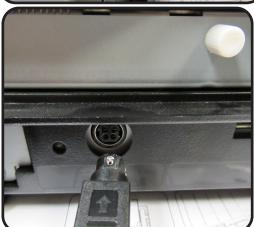
8. Slide the DS200 Scanner unto the top of the box using the tracks located on opposite sides of the illustrated instruction page. Before sliding fully back you will need to plug in the barrel power cord.
