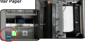
roll and reinsert it with the paper feeding under the roll coming out on the right side of the compartment. Lock and reseal the door. Reprint the report as needed.
