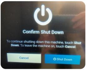
4. The unit will prompt you to "Confirm Shut Down", select Shut Down. Allow the unit to fully power off then push the rocker switch to "on" to restart. The card should eject. Enter the Election Code and complete the reopening. A new blue security seal will be placed on the access door and the manager will record the new seal number in the Incident Log.
