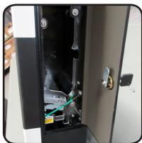
2. Open the right side panel door. If the ballot can be removed through the side, gently pull it out. Close and lock the door. If not, proceed to step 3.
