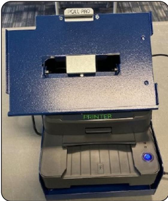
Turn on the printer by holding the power button until the blue light is on. The Poll Pad is set on the stand and held in place by the lever at the top.
